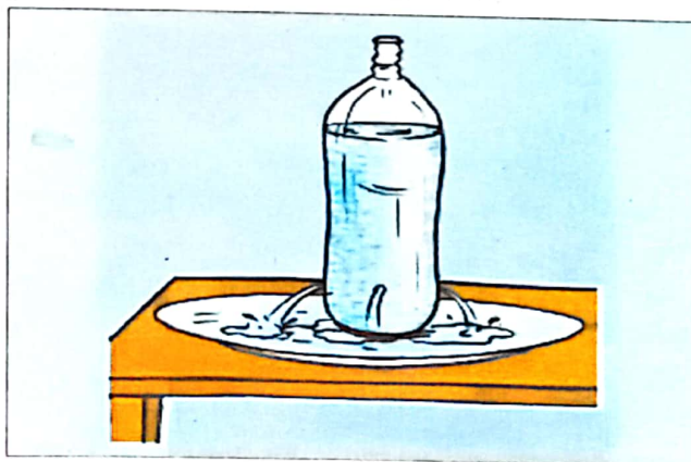
Fig. 9.16 : Liquids Exert Equal Pressure at the Same Depth
