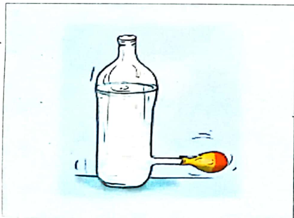
Fig.9.15 : A Liquid Exerts Pressure on the Walls of the Container
