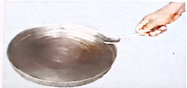
Fig. 5.4 : Vibrating Plate Produces Waves in Water
