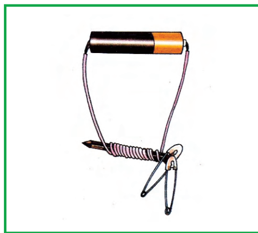
Fig.10.8: An Iron nail attracts more safety pins when wrapped with a coil with more number of turns
