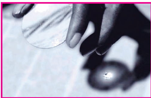
Fig.11.23: Real image of the sun by a convex lens
