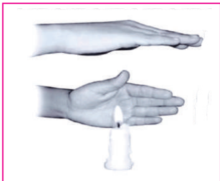
Fig.3.9 : Transfer of heat by convection in air
