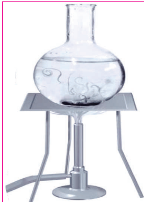
Fig.3.8: Convection of heat in water
