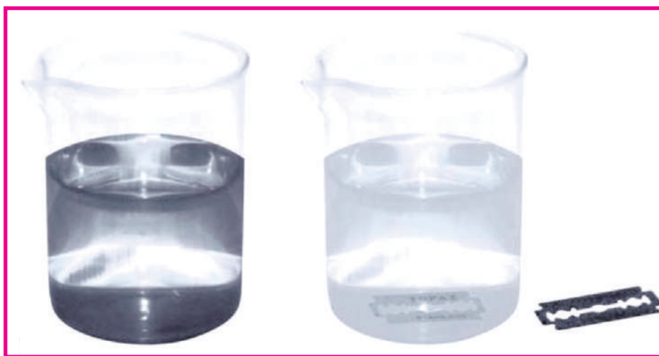
Fig.5.4: Change in colour of the copper sulphate solution due to reaction with iron
