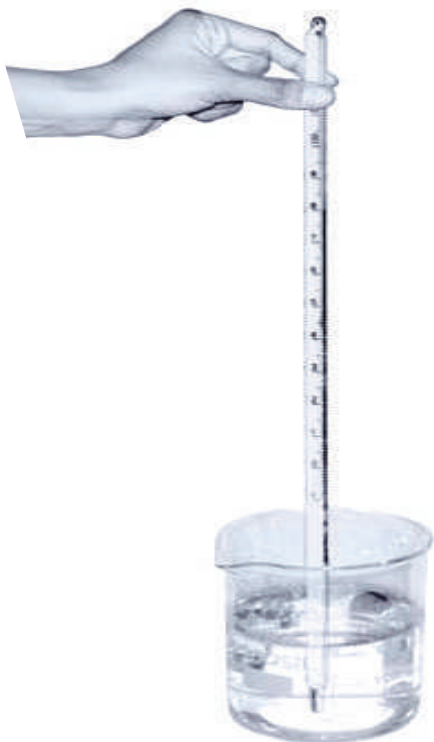
Fig.3.4: Measuring temperature of water with a laboratory thermometer
